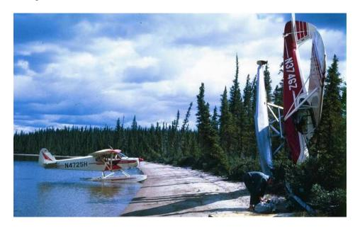
After Roger calmed down, the two pilots made a tripod from spruce trees, and with a rope sling, carefully lowered the tail. Fortunately, the Cub was undamaged except for the end of one propeller blade, which was slightly bent. But by roping a stout tree trunk to the blade and levering the tip forward, they soon had it tracking the same as the undamaged tip.
